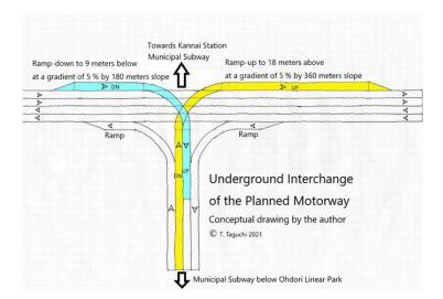
**Figure 12**. The planned interchange behind the Kannai railway station to connect Haohka canal route with Yoshida canal route (Drawing by Toshio Taguchi, with reference to MMA documents).<sup>22</sup>
