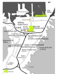
Figure 11. The initially decided plan of elevated motorway routes by MoC in 1968 (Drawing by Toshio Taguchi).
