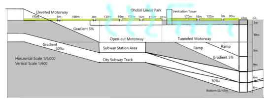
Figure 14. The coexisting subway and underground motorway along Yoshida canal (Diagram by Toshio Taguchi, with reference to MMA and Municipal Transport Bureau documents).
