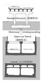
Figure 6. Change of structure from elevated to undergrounding (Drawing by Toshio Taguchi).
