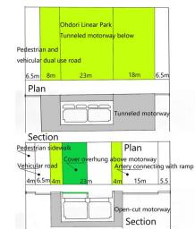
Figure 13. Plan and section of Odori Linear Park coexisted with the underground motorway (Drawing by Toshio Taguchi).
